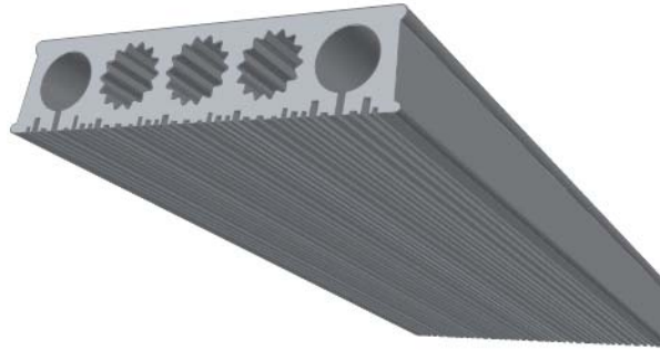
Figure 4. A hypothetical concrete floor slab. The internal and external geometry increase the functional unit by improving structural, thermal and acoustic functions. Starch foam could be used to form complex concrete forms such as these.
